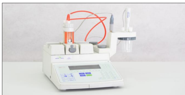
Fig 2: Potentiometric titration assembly used for NaOH delivery and pH monitoring
