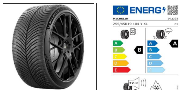
Fig 8: The Michelin Crossclimate 3 all seasons tire and its characteristics [20]
