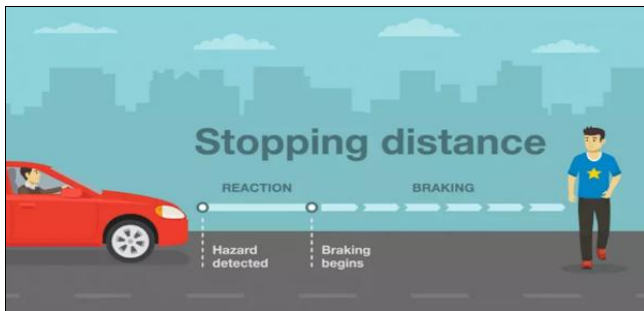
Fig 1: Graphical representation of the total stopping distance [21]
