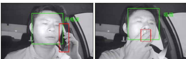
Fig 3: Driver behavior detection technology [11]
