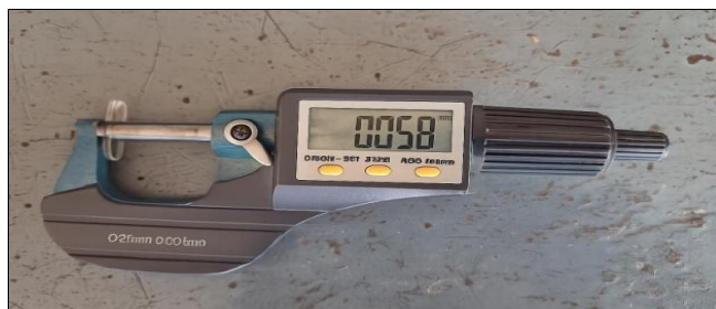
Fig 8.2: Thickness of patch
