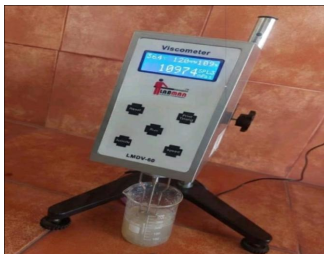
Fig 8.4: viscosity of patch
