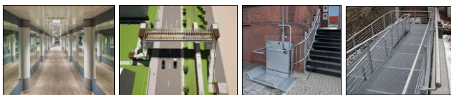
Fig 29: Underground passages (tunnels) or overpasses (footbridge) for pedestrians. Equipping them with a horizontal elevator and ramp for people with disabilities
