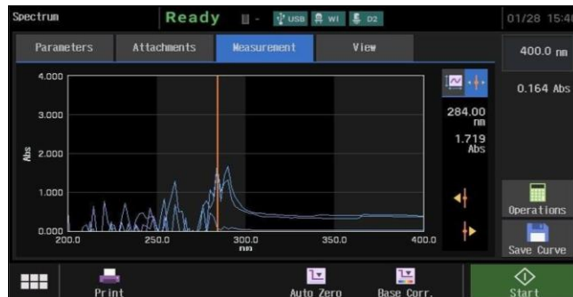
Fig 3: UV-Spectroscopy of Minoxidil
