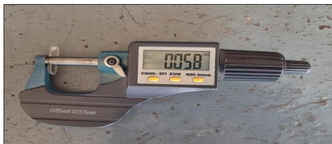
Fig 8.2: Thickness of patch
