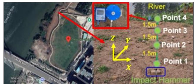
Fig 1: Ground vibration measurements conducted near the Saigon River
