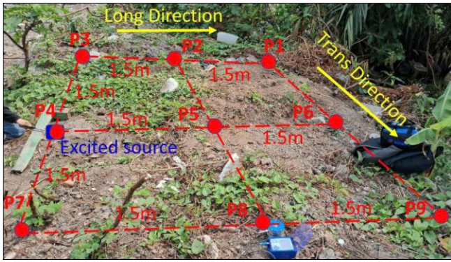
Fig 1: Experimental layout and monitoring configuration for ground vibration measurements under soil-rock impact conditions
