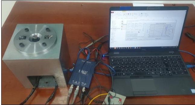
Fig 3: Frequency sweeping, impedance measurement, and resonance verification of the horn-workpiece system
