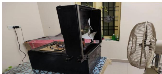
Fig 4.1.3: Testing of Hard PVC Blade
