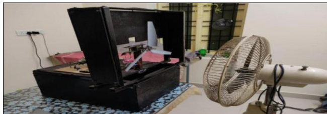
Fig 4.1.1: Testing of PVC Blade
