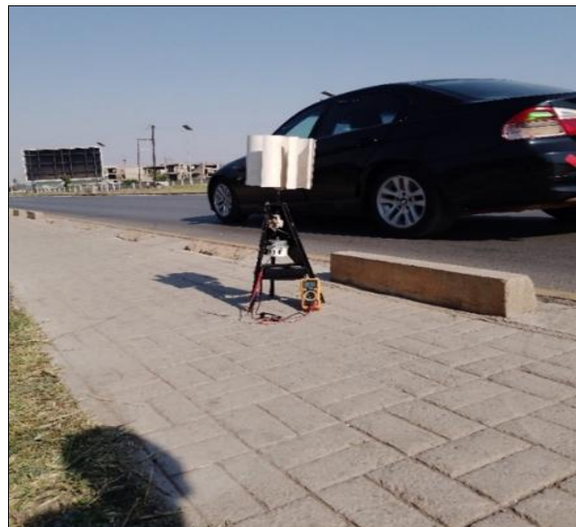
Fig 61: Turbine testing along Nangwenya road, Lusaka, Zambia
