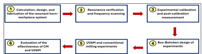
Fig 7: Flowchart of the theoretical design of the horn-workpiece system and its experimental optimization
