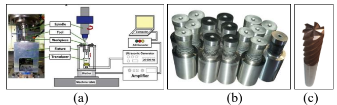
Fig 4: Experimental system, workpiece, and solid carbide end mill
