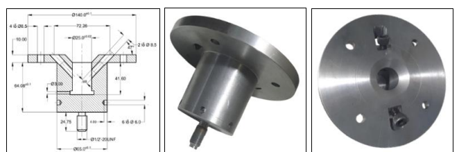
Fig 2: Design drawing of the ultrasonic horn for vibration-assisted milling
