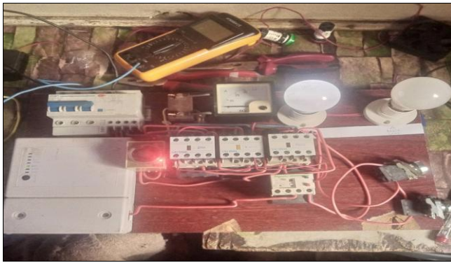
Fig 3.7: Prototype circuit operating in Star configuration
