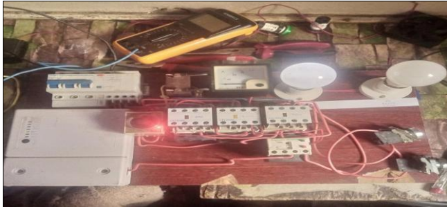
Fig 4.1: Prototype circuit operating in Star configuration
