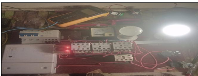
Fig 4.2: Prototype circuit operating delta configuration
