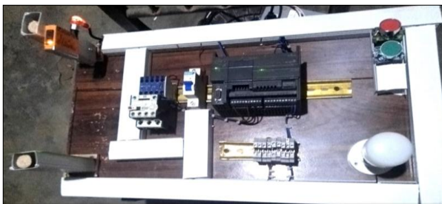
Fig 1: When the blinking LED Light is in off position when the optical sensor detects no Danger
