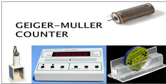
Fig 1: ST350 setup with source and GM-Tube
