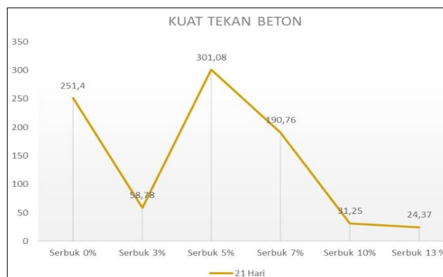
Fig 7: Graph of the compressive strength of concrete aged 21 days
