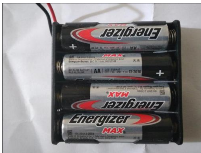
Fig 3.25: Batteries and battery holder
