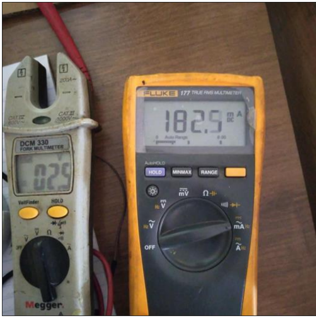
Fig 4.3: Digital multi-meters measuring current and voltage being drawn by the lighting system
