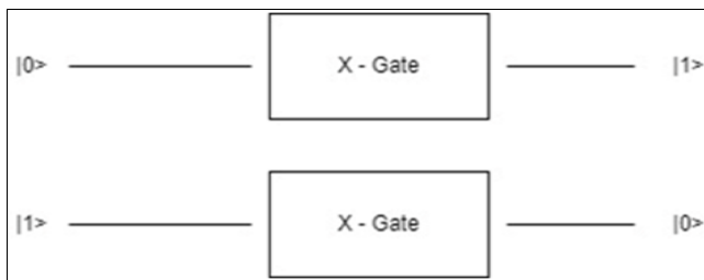
Fig 5: Optical representation of the Pauli-X gate operating in a state of a single qubit
