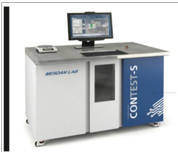
Image 1: Contest-S instrument for stickiness tester (MESDAN 2020) [32]
