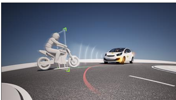
Fig 23: Autonomous Emergency Braking (AEB)/ Lane Support Motorcyclist (euroncap.com, 2024) [7]
