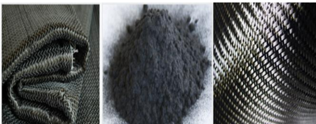
Fig 2: Different forms of CFRP
