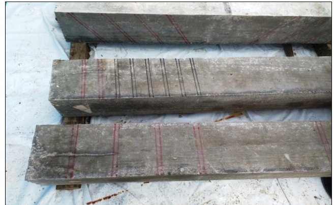
Fig 3: Marking the location of the groove
