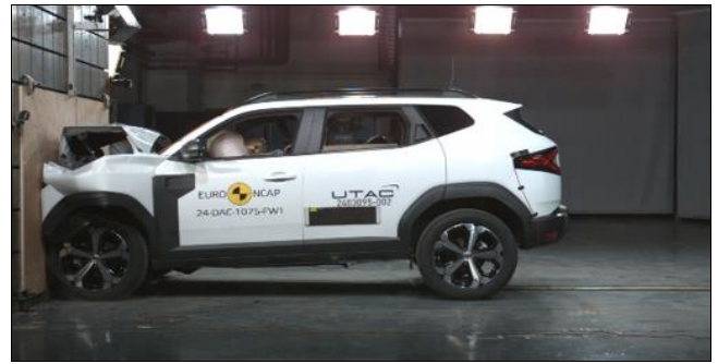
Fig 5: Dacia Duster car 3rd generation in frontal impact with an obstacle a non-deformable barrier - concrete wall [13]
