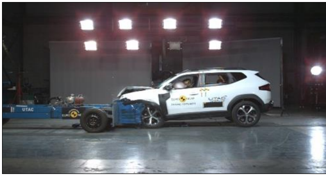
Fig 4: Dacia Duster car 3rd generation in frontal impact with an obstacle simulating a car weighing 1,400 kilograms [13]
