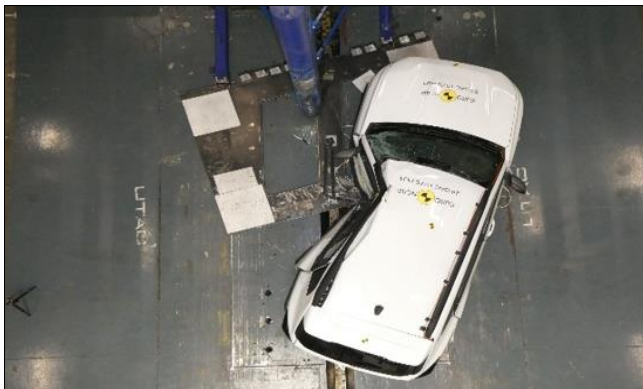
Fig 7: Dacia Duster car 3rd generation to side impact with a pylon [13]
