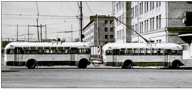
Fig 1: Trial operation of the world's first trolleybus train of two MTB-82 trolleybuses [5]
