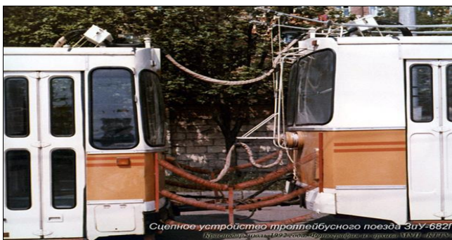
Fig 2: Coupling device of trolleybus train ZiU-682G [6]
