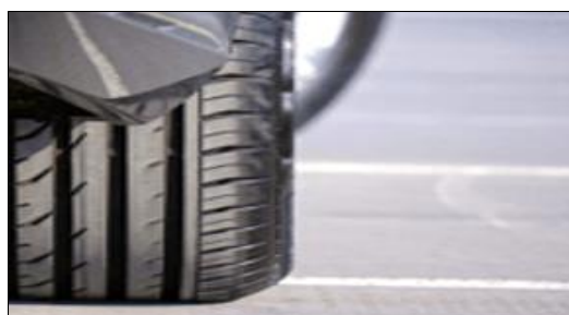
Fig 9a: Profile of a summer tyre
