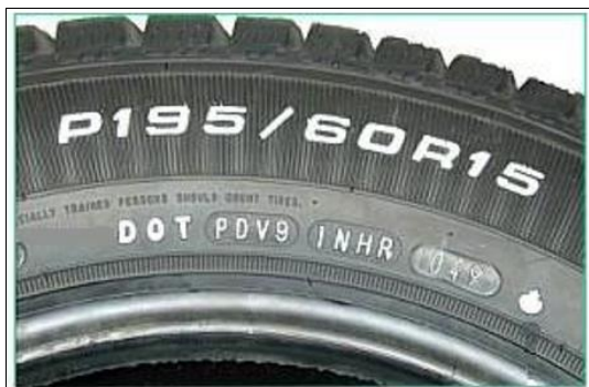
Fig 3: Markings, notations and terms specific to car tyres [3]
