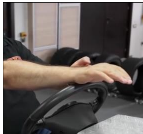
Fig 3: Adjustment of the driver's seat backrest by placing the palm of the hand with the forearm on the steering wheel [7]
