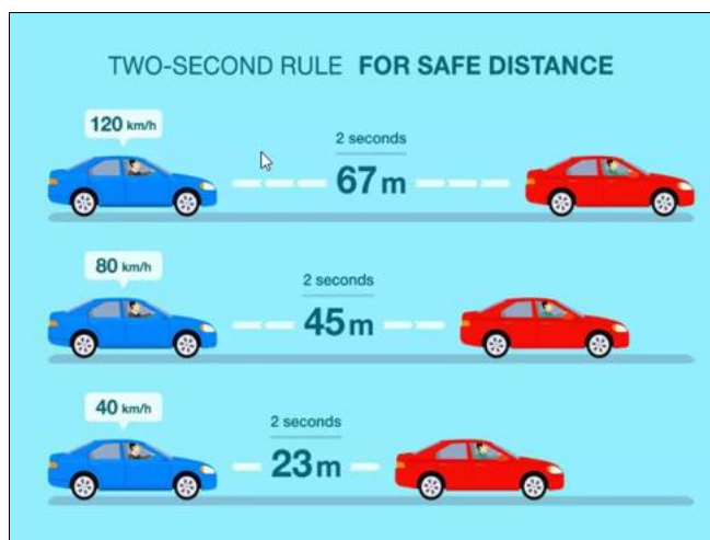
Fig 13: The two-second rule in preventive/defensive driving for safe distance [9]
