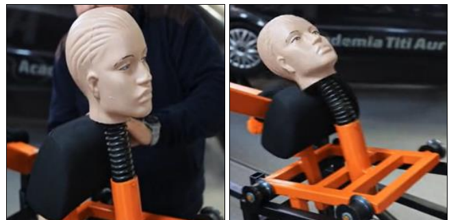
Fig 7: Inorrect adjustment of car seat headrests [7]
