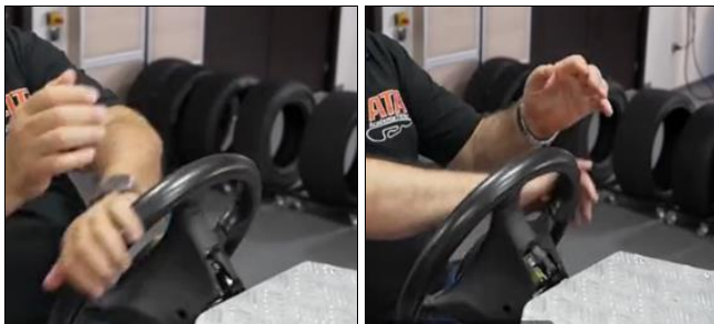
Fig 5: Correct steering wheel operation in turns [7]
