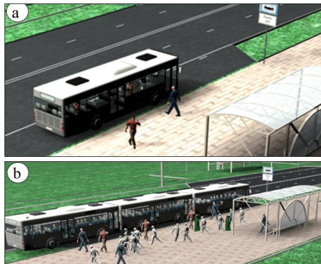
Fig 3: Use of modular PV trains with different number of modules: a - one module during passenger traffic decline; b - three modules during passenger traffic growth [35]
