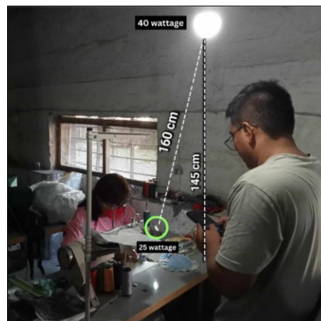
Fig 1: Shows the measurement of wattages and the area of the sewing machine from the top light
