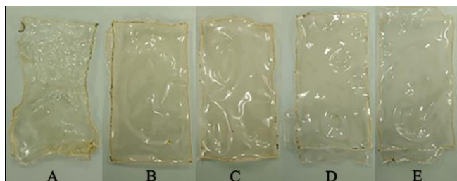
Fig 1: (A) Pure chitosan membrane; Chitosan-MMT composite membrane with (B)-0%; (C)-1%; (D)-1.5%; (E)-2% PVA concentration
