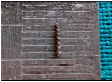
Fig 7: Retrieved instrument fragment Measured around 5 mm
